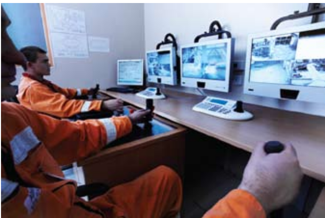
Nyrstar employees operating the blast furnace from the control room
